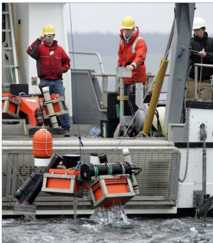
Fully rigged DT-X SUB as deployed for 5-week seafloor observatory mission.
