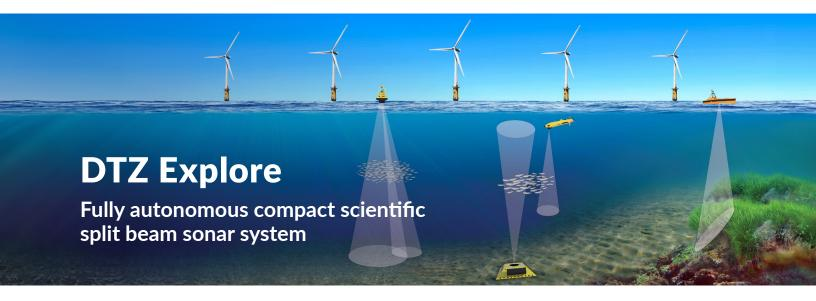
The all new DTZ Explore is the first fully autonomous scientific **split beam sonar system.** Housed in a compact, low-power, submersible unit, the DTZ is capable of long-term, full water column data collection and real-time biological event reporting.
